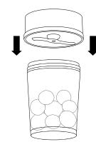
2. Place cup onto the base. The unit is now powered and in Standby mode with the Power LED illuminated. Press desired speed. When done chopping, press the activated speed to stop.
